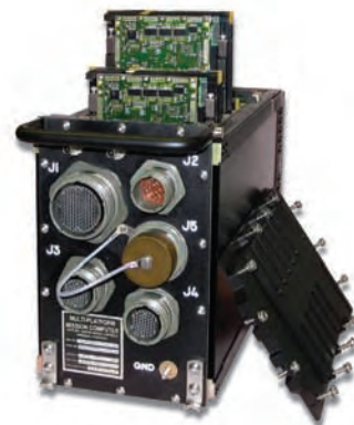
One of Curtiss-Wright's innovative family of PCOTS subsystems, the MPMC 350p houses up to 3 rugged DCP-124 PowerPC SBCs, Ethernet, Serial and DIO interfaces.
