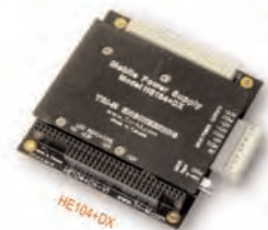
108 Watt PC/104+ Power Supply
